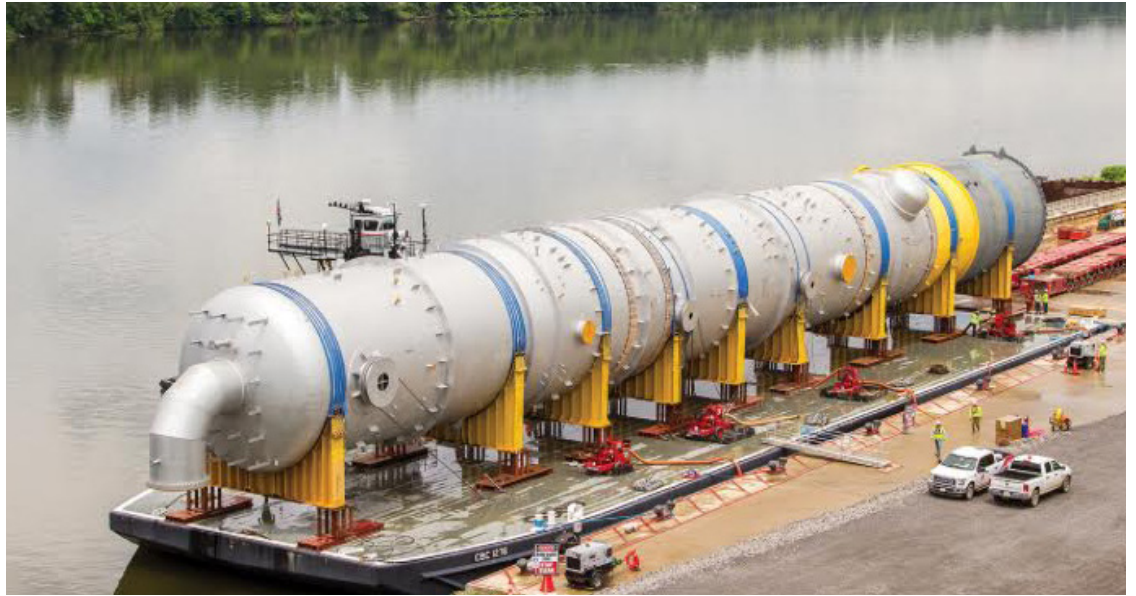
The M/V Big Eddie of Crosby Marine is seen at Monaca, PA, Mile 27.9 on the Ohio River, on May 30 with a deck barge carrying a large refiner vessel for the Shell Oil Corporation ethylene cracker plant under construction near Pittsburgh. Pictured here are pumps used to level the Canal Barge Company barge for unloading, and the heavy-duty flatbed carrier to transport equipment to the construction site. Photo by Eric M. Johnson, Waterways Journal
