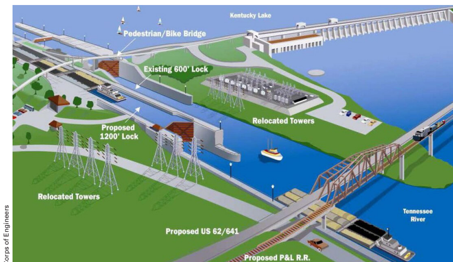
The Kentucky Lock Addition Project, Paducah, Ky., includes design and construction of a new 110'x 1,200' lock to be located landward of the existing 110'x 600' lock.
