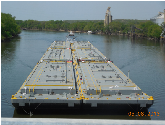
The company's newer tank barges have 6psi tank tops, heavy hull scantlings, and stainless steel external fittings.
