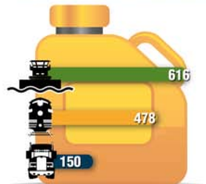
Ton-miles Traveled per Gallon of Fuel
